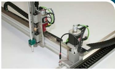
Utilises our traverse system to position the profiler in a 2D or 3D environment
