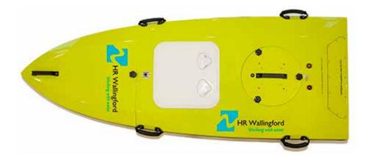
The ARCboat is a remote controlled boat that is used to collect river and estuarine data including flow, depth and suspended sediment concentrations.
